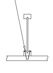
To minimize splitting of flange and bearing plate, angle nails and start at least  $1 \frac{1}{2}$  from end.
