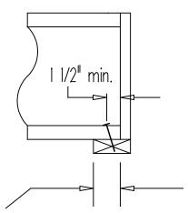
1 3/4" minimum end bearing length for all floor \$ roof details. Longer bearing lengths may be indicated on the placement plan.
